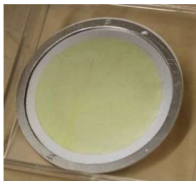
99.934% ^{235}\text{U} 363 \mu\text{g cm}^{-2} ^{235}\text{U} laag door "molecular plating" Laag \varnothing : 42 mm Substraat: 0.03 mm Al
